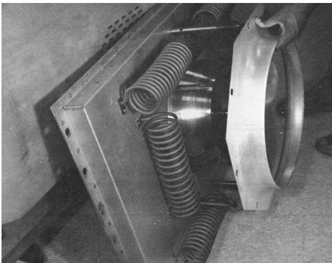
Figure 78 Fan shroud removed
