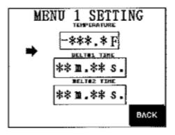
6. To set the temperature press on the temperature setting, opening the keypad for changing it. Enter the new temperature and press ENT.
